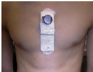
Figure 1 The R-R interval, posture and activity recording device attached on the center of the chest with three disposable ECG electrodes. The device is 5 x 13 cm, the thick is 1 cm and the weight is 30g.
