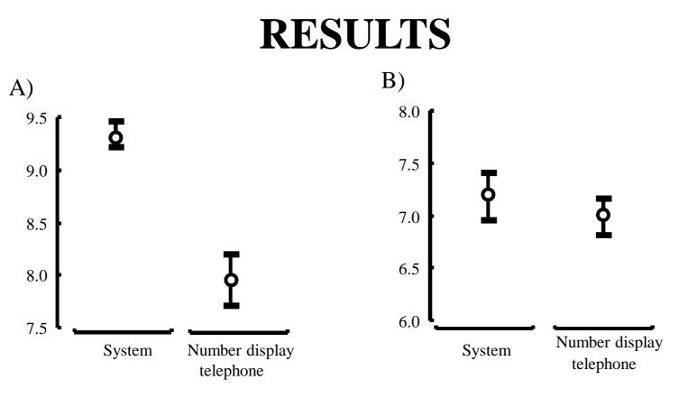
The connection times from the system to the conventional phone and from number display phone to the conventional phone (plot A). The connection times from the conventional phone to the system and from the conventional phone to the number display phone (plot B).
